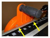
• You have to detach the cutting head by unscrewing the knob securing the head against one of the column of the machine.
