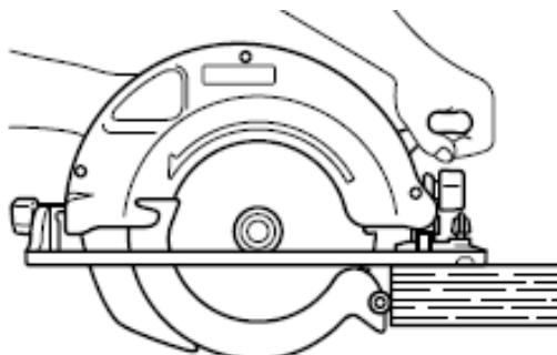
G) Switch the tool on and wait a couple of seconds until the saw blade movement reaches operating speed. Slowly, with slight pressure on the tool, drive the saw blade into the surface of the workpiece. When you finish cutting or move the saw away from the workpiece, the movable saw blade guard closes automatically.
