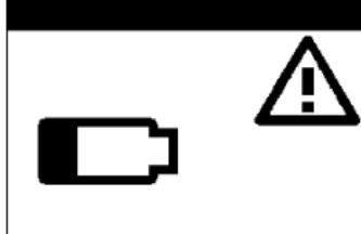
If the indication shown here appears in the display, the batteries must be replaced. Measurements are no longer possible.
